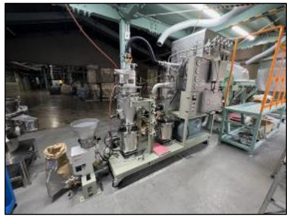
[エア分級設備]
