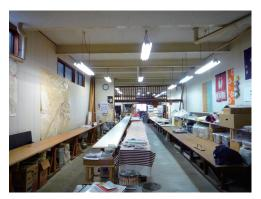
One 12- to 13-meter bolt of cloth can be dyed on a single board set up in the middle of the plant
