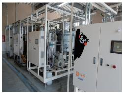
The factory's four reduced-pressure distillation units, which enable about 3,000 liters per day of BDF to be produced
