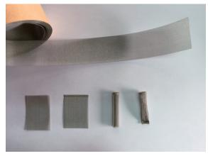
Wire mesh used as a material for filters, which is processed by means of manual operation
