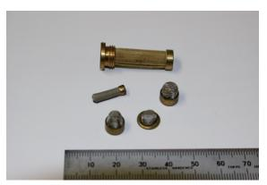
A finished automobile filter; mechanization of the process is difficult due to the need for microfabrication
