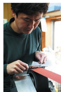
Manufacturing scissors by hand, relying on both experience and intuition
