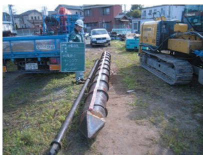
Experimental prototype of small casing that is one-tenth the regular size
