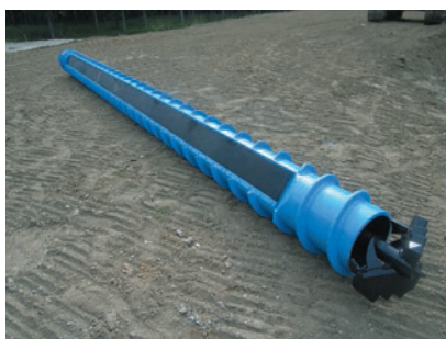
Casing that allows pouring of crushed rock from the side
