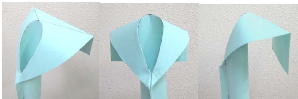
図1-1-4 Forming collar with packaging seam
