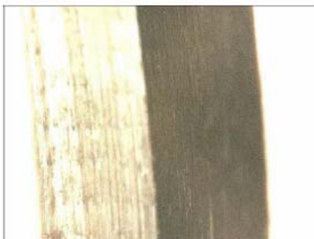
Fig.4-1-3-2 TR20 切削加工ねじ x 100 倍
