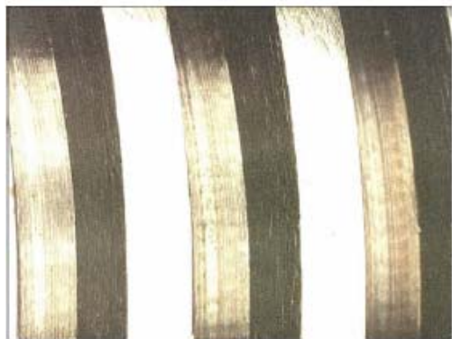
Fig.4-1-3-1 TR20 切削加工ねじ x 30 倍
