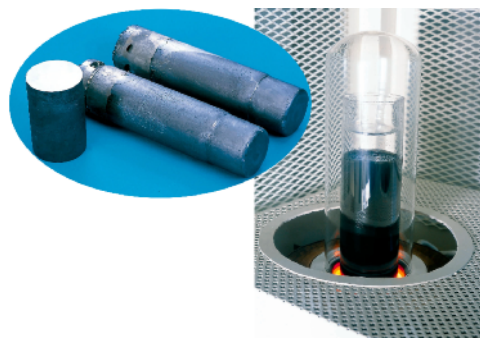
CdTe single crystal ingot (in circle) and the crystal growth furnace
