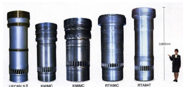
Completed cylinder liners
