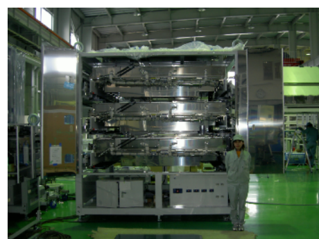
Heating equipments for the 8th generation
