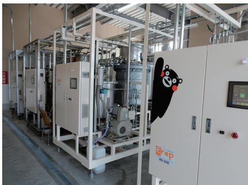
The factory’s four reduced-pressure distillation units, which enable about 3,000 liters per day of BDF to be produced
