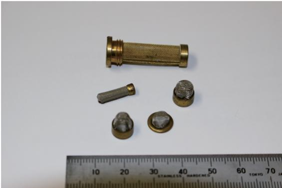
**A finished automobile filter; mechanization of the process is difficult due to the need for microfabrication**
