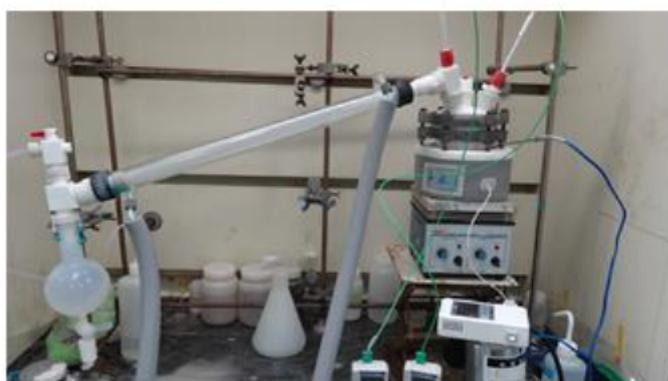
Simple distillation apparatus made of PTFE
