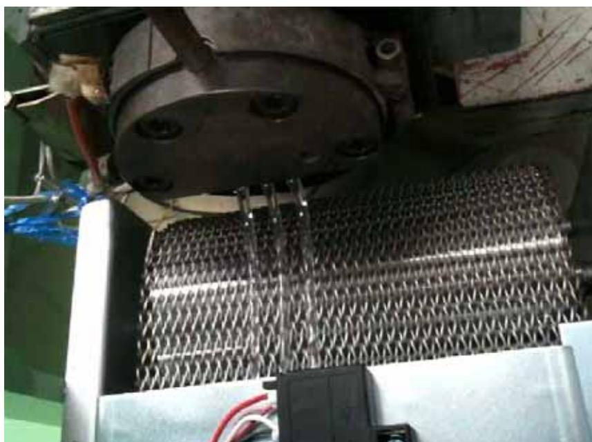
Fig.3-1 Photographs of RPET strand at compounding machine.
