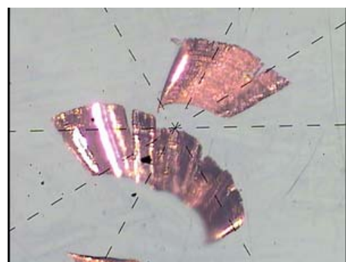
Fig2-2-2-5 顕微鏡写真-切粉 ×50
